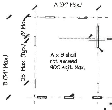
Provide drag struts consisting of blocking with steel strap or joist in line with wall line with strap to top plate of wall
